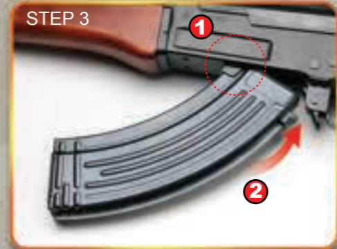
1. First locking the front of Magazine. 2. Locking the rear of Magazine until you heard it click into place. The gun is ready to fire.
